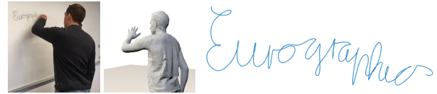
Figure 11: SIP is capable of recovering the handwriting on a whiteboard. Left figure: image of the writing scene, middle figure: recovered pose at the end of the handwriting, right figure: recovered wrist motion projected on the whiteboard plane.
