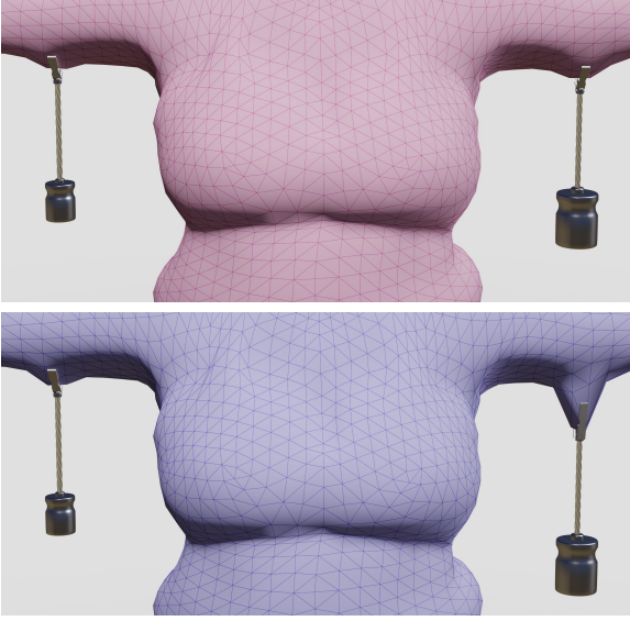
Figure 5: This picture shows the deformation of our material (top) in comparison with the nonlinear flesh material defined in [SGK18] (bottom), for two different weights under gravity: 0.5Kg (left) and 2.0Kg (right). It can be clearly seen that our material provides a higher nonlinear response.
