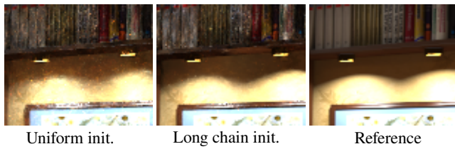
Figure 6: Comparison of different chain initialization procedures with the same number of initial samples. Left: Using only a limited number of uniform samples to select the initial state cannot ensure that the initial state is selected according to the target function, which results in visible bias. Center: Our method uses on a properly initialized global MCMC chain to perform initialization of many chains, reducing the start-up bias.
