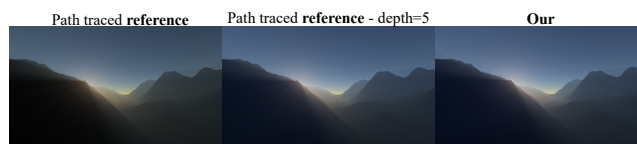
Figure 14: Volumetric shadows from the atmosphere, from left to right: path-traced single scattering, path-traced multiple scattering (depth = 5) and our real-time approach using ray marching and cascaded shadow maps.
