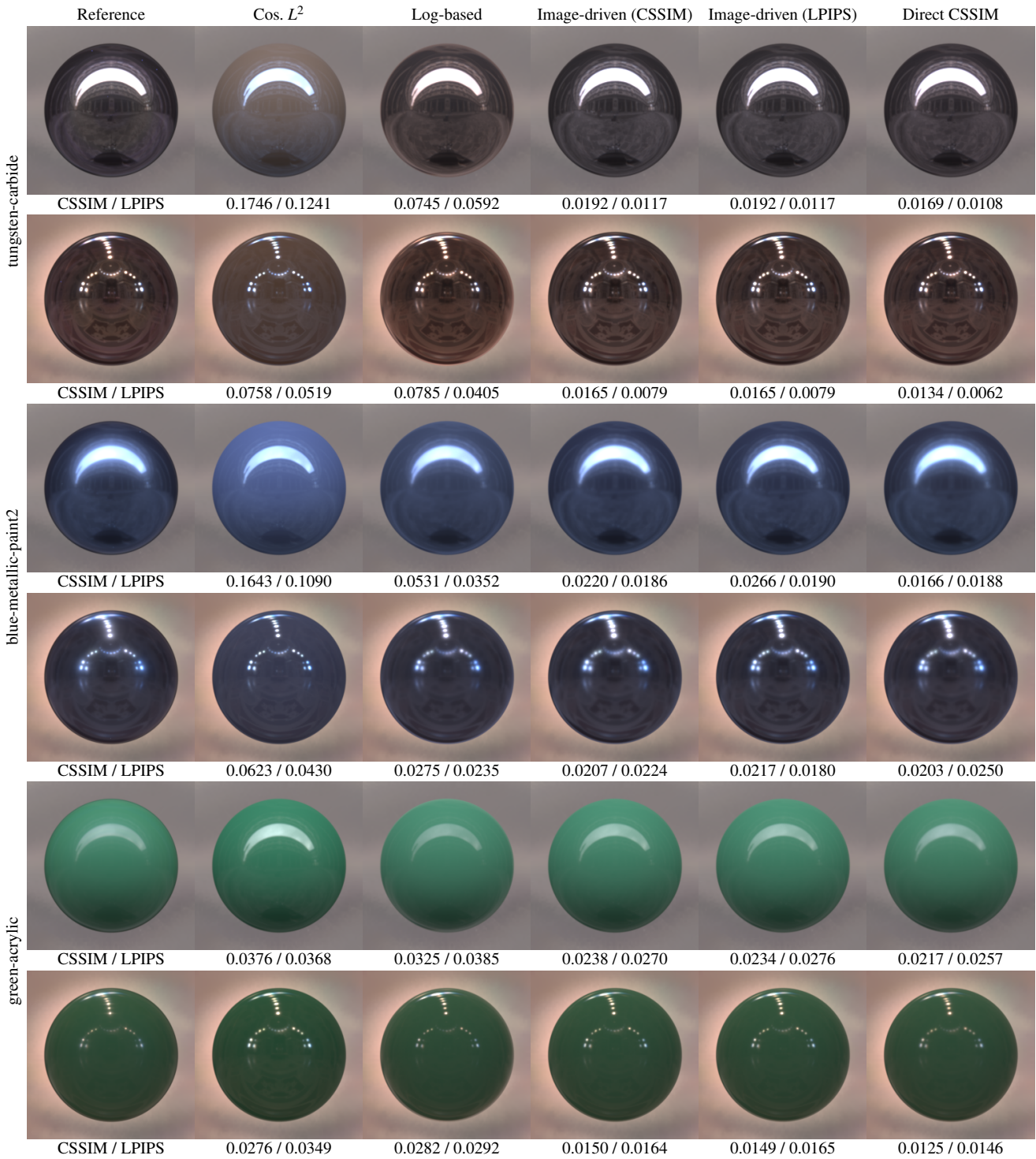
Figure 4: Image-driven BRDF fitting on three selected materials with the GGX microfacet BRDF model compared to the classic cosine weighted L^2 BRDF fitting metric and Löw et al.'s log-based fitting metric. The CSSIM and LPIPS error is shown below each BRDF fit visualization. Note that the “Direct CSSIM” results are optimized to produce an as low as possible CSSIM error under the lighting shown. Hence it represents a lower bound on the CSSIM error for each material under the shown lighting.
