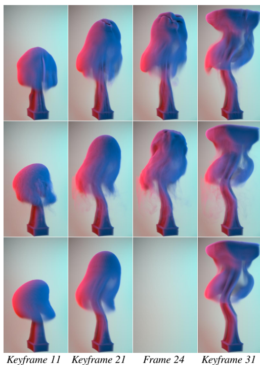
Figure 10: 3D twist example at resolution 100 \times 200 \times 100 . The method of Baseline (top row) does not precisely match target keyframes (bottom row). Our method (middle row) generates smooth transitions and matches target keyframe well.
