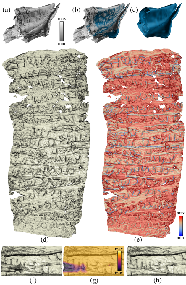
Figure 8: Silver scroll: (a) volume rendering of \mu CT image; (b) same as (a) with M_{curv} ; (c) M_{curv} ; (d) thin iso-surface rendering; (e) thin iso-surface rendering with distance to M_{curv} color-coded (blue=behind, red=in front of M_{curv} ); (f) zoom-in with occluding structure; (g) modified ray length color-coded; (h) occluding structure partially removed.
