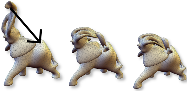
Figure 5: An elephant deforms as its trunk is pulled downward toward its body, undergoing collisions with the tusks and ear. Intermediate iterations of the simulation are shown with and without constraint removal (center and right, respectively). When constraints are not removed, visible sticking occurs between the trunk and tusk, motivating the need for a dynamic constraint set.
