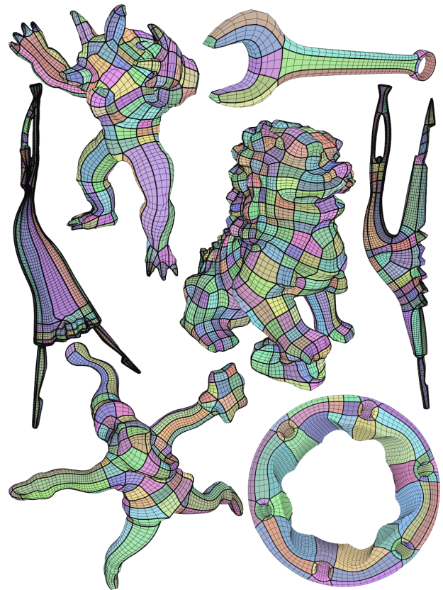
Figure 7: Our method's result layouts and meshes on various models with cross field derived input singularities.
