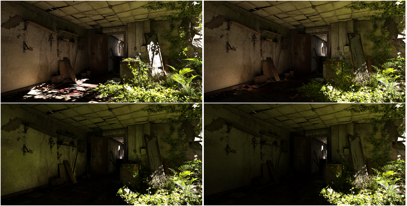
Figure 11: Sample validation can effectively suppress bias caused by temporal reuse in dynamic scenes. Top left: original lighting. Top right: without sample validation, visible bias still remains after 12 frames of sudden change of sunlight—note the illumination on the wall on the left. Bottom left: with sample validation, the result rapidly adapts to changes in lighting. Bottom right: converged result.
