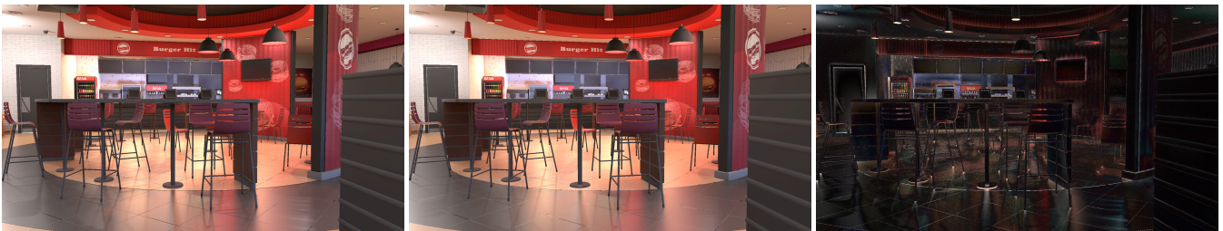
Figure 9: Bias caused by spatial reuse. Left: Unbiased result. Middle: Biased result. Right: 10\times difference. Note that bias is mainly in shadow areas due to visibility changes. The glossy floor worsens bias around the chair legs because the target function includes glossy reflection and tends to place more samples around the specular reflection direction.
