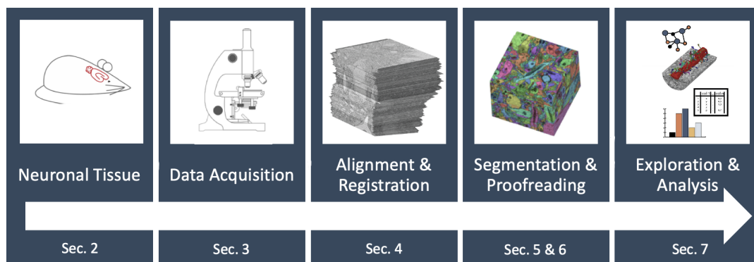
Figure 1: The connectomics pipeline: In this survey, we discuss visualization approaches for each step of the connectomics data processing pipeline. Visualization is not just important for the final analysis step but vital for efficient image acquisition, registration, segmentation, and proofreading of segmentations.
