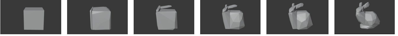
Figure 6: Morph stages of the collision shapes for transferring the cube motion to a bunny after applying V-HACD.
