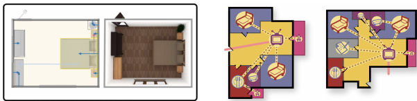
Figure 5: Neurosymbolic layout generation via learning to synthesize layout constraint programs. Left: A graph neural network synthesizes a constraint graph specifying furniture spatial relationships; a neurally-guided search then finds object placements that satisfy those constraints [WLW*19]. Right: A transformer + pointer network architecture synthesizes a floor plan layout constraint program, which is then solved to produce a floor plan [PGK*21].
