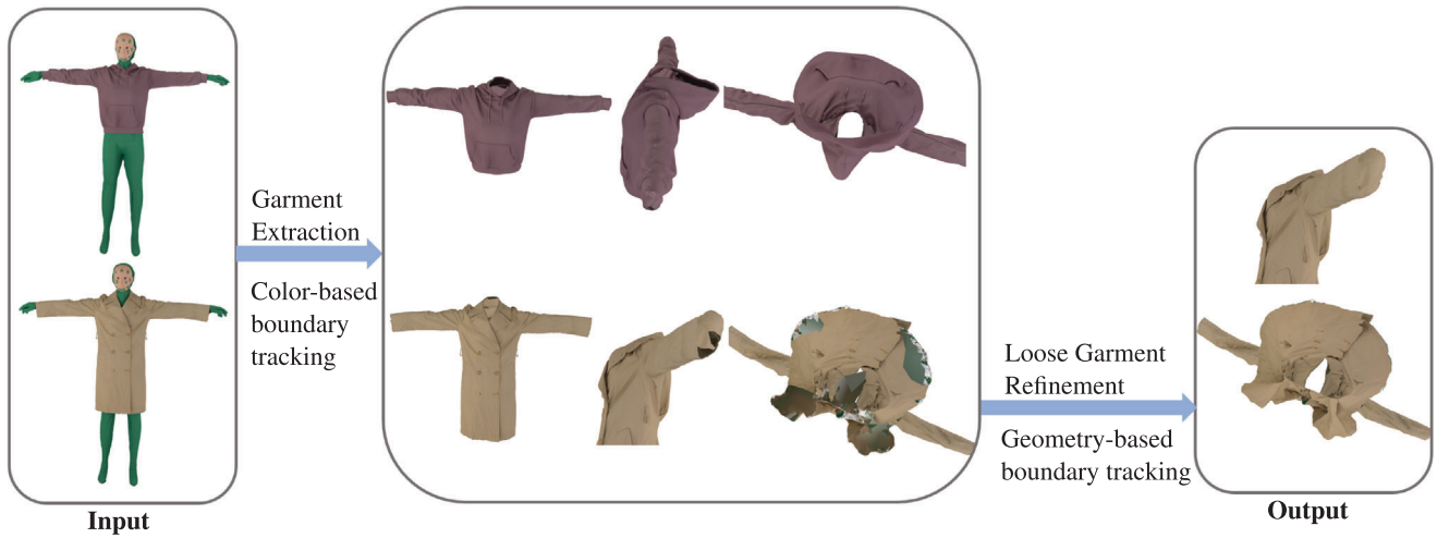
Figure 1: Our method can handle both tight and loose garments. Given a 3D scan of a clothed mannequin, our system extracts a garment mesh by colour-based boundary tracking, and then automatically categorizes the garment into tight or loose. For a loose garment, geometry-based boundary tracking is executed to refine the extracted mesh.
