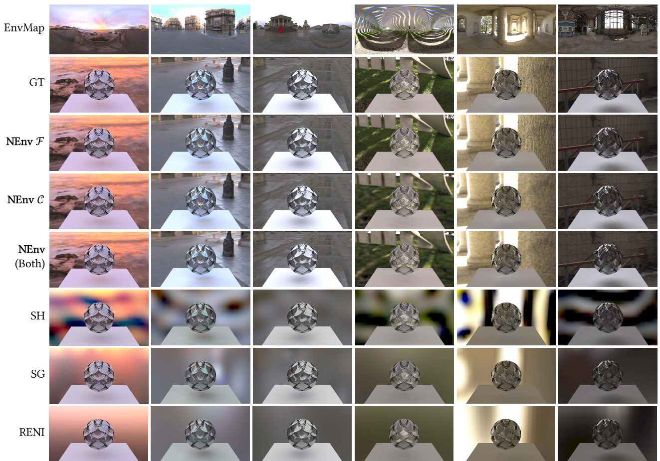
Figure 9: Render comparisons of different configurations of our work with the ground truth environment map and previous work, rendered at 2048 spp. Best viewed in color on a screen. Please zoom in for details.
