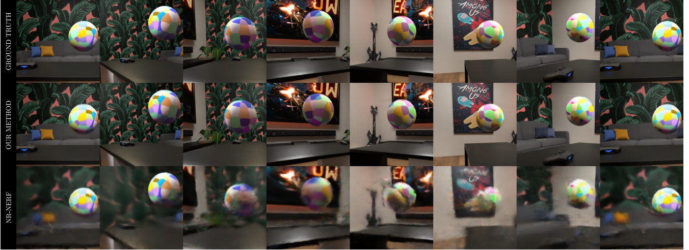
Figure 7: Motion reconstruction for the same sequence as Fig. 3 using NR-NeRF [TTG*21]. First row is ground truth, second row is our method and third row is the output of NR-NeRF. Our method can capture higher-quality motion and geometry.
