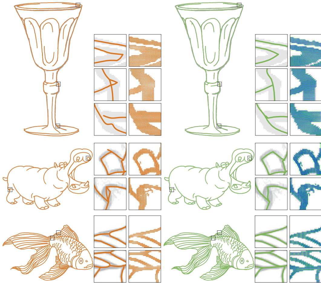
Figure 8: Compared with the results of Polyvector Flow by [PNCB21] with their original frame fields (left, orange/brown), using our frame field design with their tracing method can substantially improve the final result (right, green). Since we kept the tracing method as is, all the improvements are solely due to the absence of singularities and higher overall quality of the frame field. Inputs from https://www.easy-drawings-and-sketches.com/ ©Ivan Huska.
