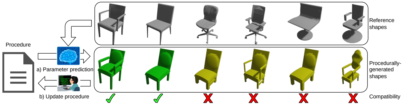
Figure 2: Overview of our data-guided authoring of procedural models. (a) The system predicts procedural model parameters for reference shapes, and estimates the compatibility between procedurally-generated shapes and reference shapes. (b) The user manually updates the procedure to improve shape compatibility.
