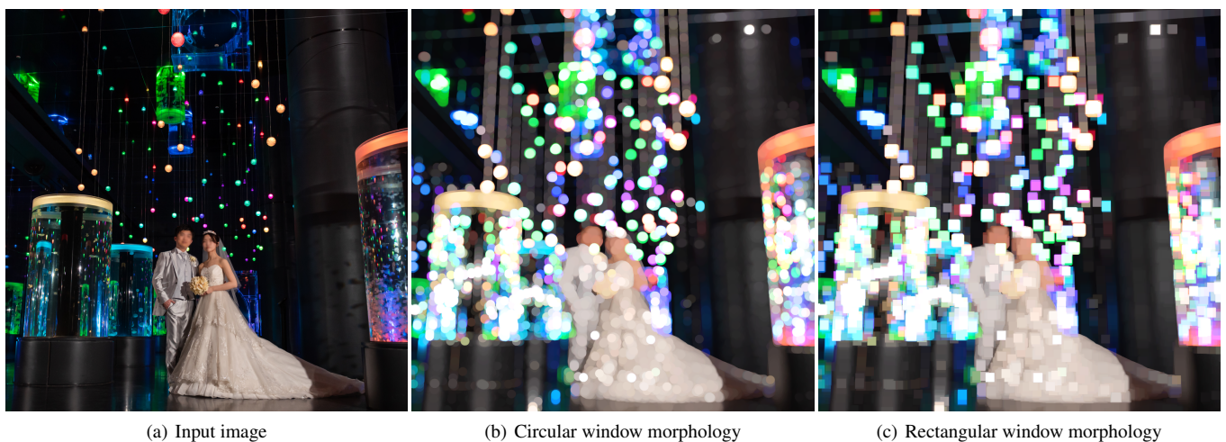
Figure 1: Example of a bokeh filter using dilation, a type of morphological operation. By filtering at the maximum value within the circular window, highlights are enhanced, creating a beautiful expression that differs from actual lens blur. As a blur effect, circular windows are typically preferred over rectangle windows due to their isotropic feature.
