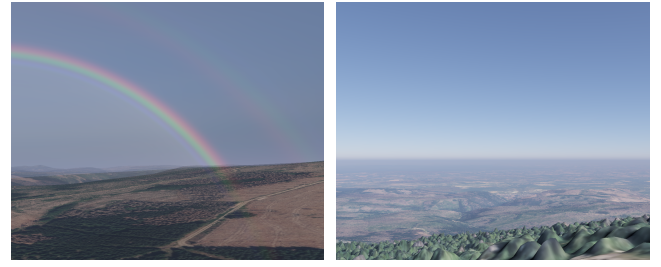
Figure 7: These screenshots show weather conditions generated by different parametrizations of the aerosols. Particles with about 0.1 mm radius and the refractive index of water result in beautiful rainbows. The right image shows a dense layer of haze close to the ground. To simulate this, we used a custom density distribution with a constant density up to an altitude of 700 m followed by a quick exponential falloff. A photograph of a similar situation can be seen in Figure 2.
