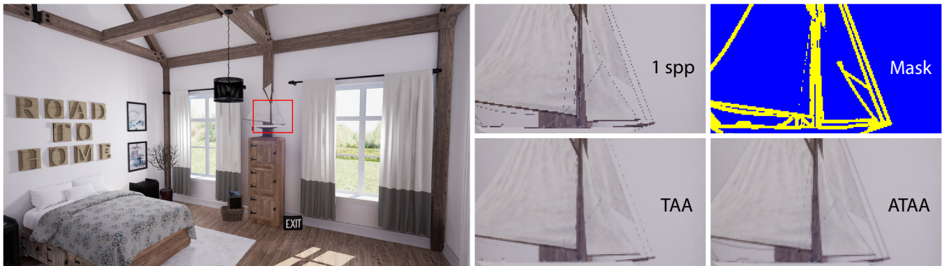
Figure 1: A modern house scene in Unreal Engine 4 with deferred shading, ray traced shadows, our adaptive temporal antialiasing technique, and a moving camera at 30 fps on NVIDIA Titan V. Zoomed details show raw 1 sample per pixel raster input, standard TAA output, a visualization of our segmentation mask, and our ATAA 8x result.
