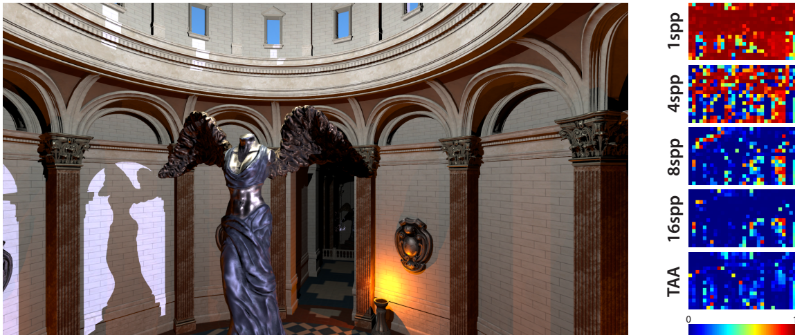
Figure 1: We use a deep classification network to detect aliasing artifacts in image sequences. In this example we show the output for one sequence of 4 frames. The network generates a scalar value as a measure of aliasing for each 64 \times 64 tile of this sequence, resulting in the images shown on the right. Increasing sample counts result in lower overall output. Further, since we only measure aliasing, use of high-quality temporal antialiasing (TAA) correctly results in output similar to that of 16spp images. Metrics like SSIM and PSNR would classify the former as being much different from the latter.
