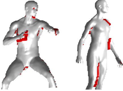
Figure 2: Inaccuracy of the scanning device and suboptimal measurement conditions often result in structural instability of the acquired data. This is usually manifested as the topological merging of neighboring parts of the surface mesh (marked above in red on simulated rangemaps) and missing parts [CRB*16].
