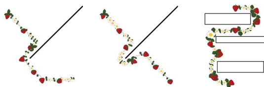
Figure 9: Path planning around obstacles. Minimizing just the geometric path length makes the ornament avoid the obstacle (black line), but the path follows the obstacle’s shape only on the upper side (left). We prefer it to follow it on both sides, which we achieve with modified edge costs that pull the path towards the straight line between the endpoints (center). The path is pulled in between the lower obstacles, aligning the path better to the obstacles (right).
