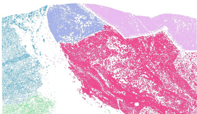
Figure 4: Clustering of a LiDAR point cloud according to the canopy color, aimed at differentiating tree specimens.
