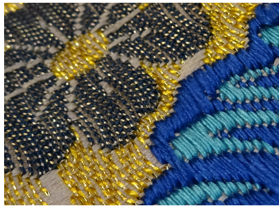
Figure 4: Detail of an historical fabric weaved in silk and metallic yarns (golden ones)
