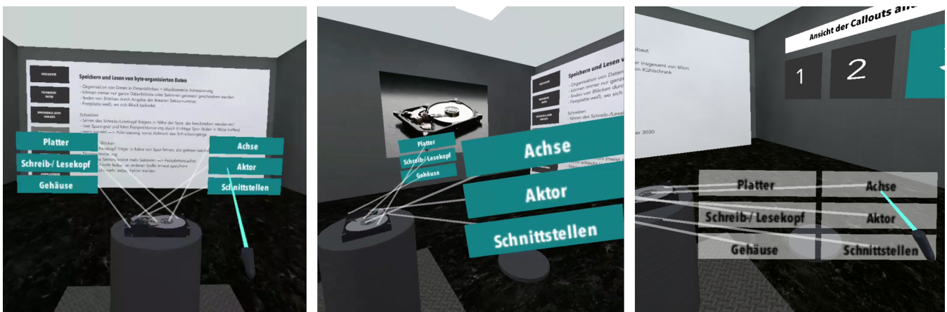
Figure 1: Three alignment-types of callouts in a virtual reality application; Left: Static callouts oriented in one specific direction. Middle: Static callouts that keep an orthogonal orientation towards the user. Right: Head-up display callouts that move with the view of the users view.
