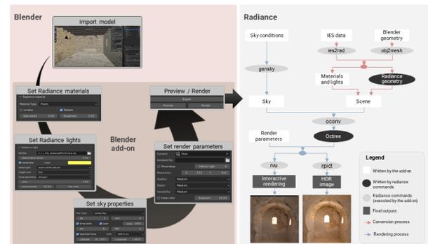
**Figure 1:** Workflow of our tool: the user configures the simulation through menus, and our add-on automatically handles data conversion and Radiance commands' execution to get the final image.
