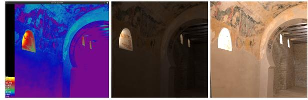
**Figure 2:** Our add-on produces light measurements on the surface (left) and HDR images (low-key, middle; high-key, right).
