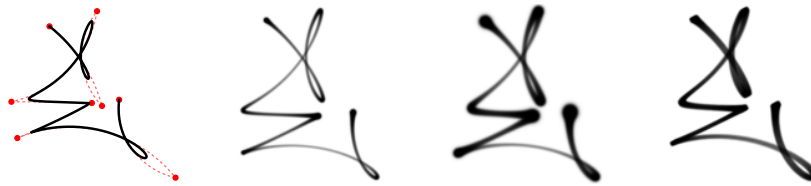
Figure 1: Sigma Lognormal trajectory, the corresponding action plan (in red) and renderings with different kinematic dependent brushes.
