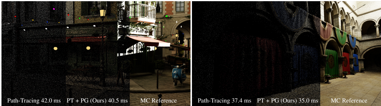
Figure 1: Frames of the Bistro scene (left) and the Sponza scene (right) with complex light scenarios are rendered with 1 spp using Path-Tracing (PT) and our Path-Guiding (PG) solution, and also with 2048 spp for reference. Notice the decrease in overall noise level for diffuse and specular surfaces, the ability of our algorithm to capture high-frequency indirect shadows just relying on 1 spp. Also, there is a slight performance boost. The images were rendered at 1080p resolution on a high-end desktop machine with RTX 2070 using the Falcor framework [NBW20].
