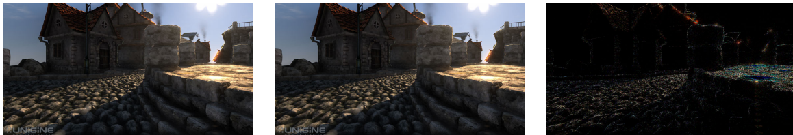
Figure 1: Left: a frame from Heaven 3.0 running in our simulator, i.e., a ground truth image. Center: using our pixel merge unit, the resulting image is nearly identical to the ground truth but with about 12% less shading. Right: scaled difference (100×) between the left and the center. With higher tessellation settings for this frame, the reduction in shading goes up to about 15%.
