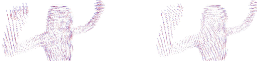
Figure 6: Left: result for the Lucas-Kanade method. Right: result for the Horn-Schunck method.
