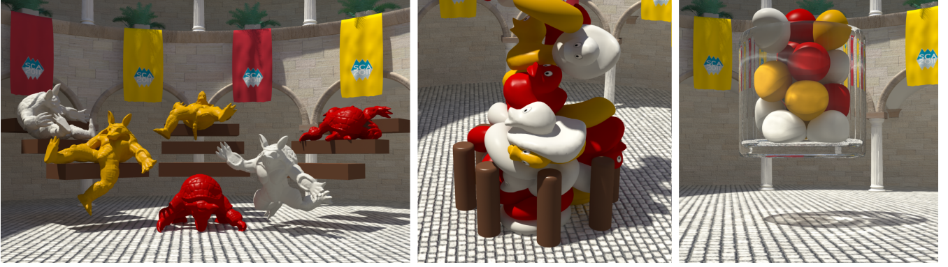
Figure 25: Robust and volume-conserving deformations using shape matching. Armadillos (32442 particles total), 20 ducks and 20 torii (21280 particles total) and 20 balls (7640 particles total) were simulated in real-time on a GPU.
