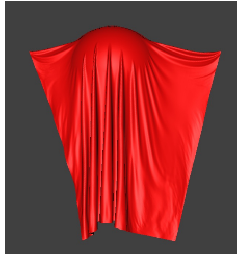
Figure 15: Simulation of a piece of cloth with 90K vertices at 20fps on a GPU using LRA.
