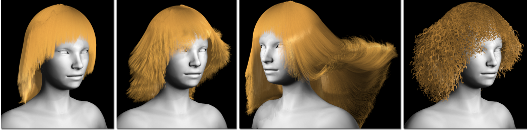
Figure 16: Dynamic FTL allows the simulation of every hair strand in real time. From left to right: 47k hair strands simulated at 25 fps including rendering and hair-hair repulsion. Long hair composed of 1.9m particles at 8 fps. Curly hair using visualization post-processing.
