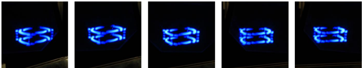
Figure 8: The 3D cuboid wireframe image (50 mm in width, 40 mm in depth, and 20 mm in height and rotated 15 degrees around Y-axis shown in Figure 6.) (Left) View from 10 degree left. (Center left) View from 5 degree left. (Center) View from the center. (Center right) View from 5 degree right (Right) View from 10 degree right.
