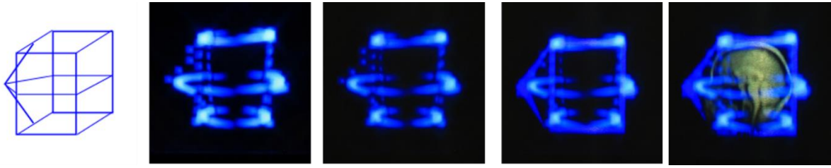
Figure 11: The 3D human head model image and its 2D cross-sectional image projected on the silk screen. (Left) 3D human model image composed of a cuboid, a leftward arrow, and a pentagon. (Center Left) Constructed 3D wireframe image from front view. (Center) A 3D image in which the silk screen is inserted. (Center Right) Superimposed 2D cross-sectional blue image of the wireframe. (Right) Superimposed 2D brain image inside the 3D head image.
