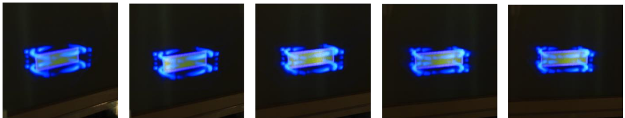
Figure 10: The 3D image and its 2D cross-sectional image projected on the silk screen.
