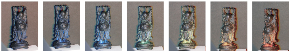
Figure 11: We sprayed the retro-reflective coating on a fabricated 3D object. When the projector array projected various solid colors (rainbow colors) from each projector, we could observe individual colors at different viewing angles.
