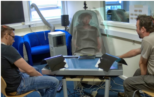
Figure 5: View of the remote confederate between the participant (LHS) and the co-located confederate. Cross-talk between the spatially segmented views is apparent.
