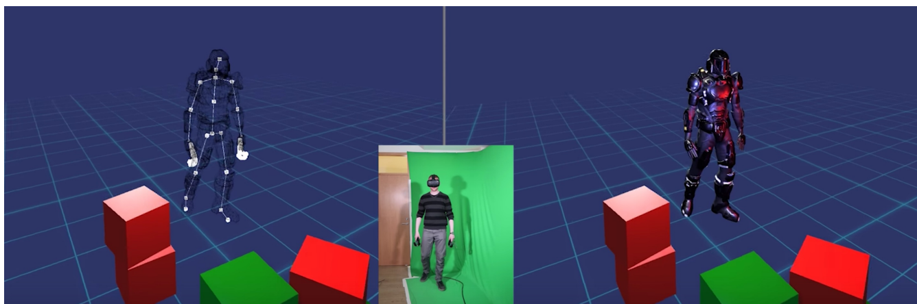
Figure 1: Full-body user motion mapped to a first-person avatar, integrating data both from an HTC Vive and a Kinect V2.
