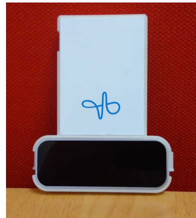
Figure 1: The Google Soli (top) and Leap Motion (bottom) devices can both detect micro-gestures.
