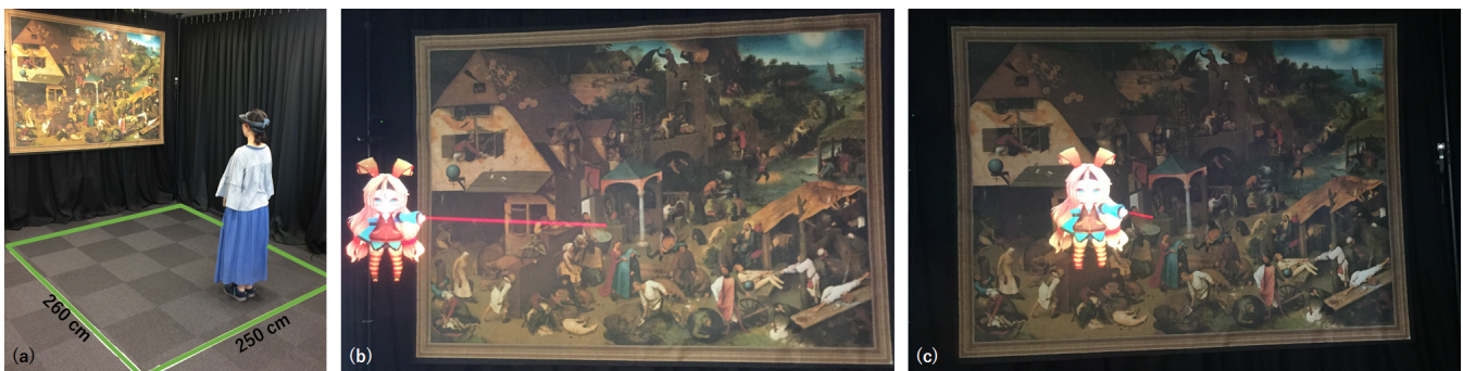
Figure 1: Images of the experiment setup showing (a) the area in which the experiment took place and then the actual view through HoloLens with (b) Outside type and (c) Inside type position interfaces.
