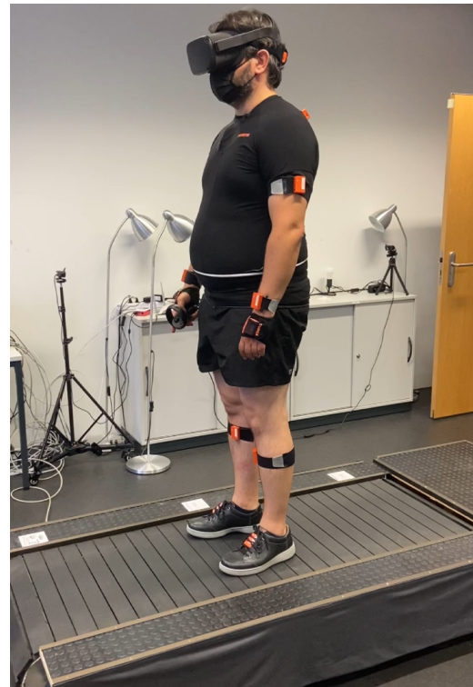
Figure 2: Test subject with Oculus Quest VR headset and Xsens motion capture suit on the PPS55 med
