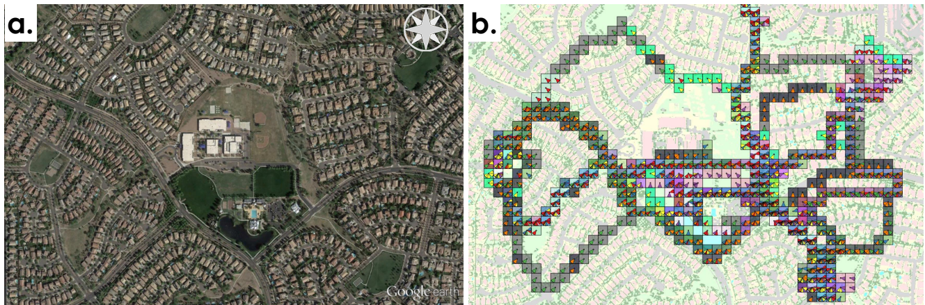
Figure 3: Coloring a map according to glyph similarity to highlight zones of similar microclimate. (a) shows the physical structure of the study site (Google Earth, 2015), while (b) shows the colored grid cells and the corresponding glyph distribution (background map: [Env12], see Fig. 1a for the meaning of a glyph segment's color).
