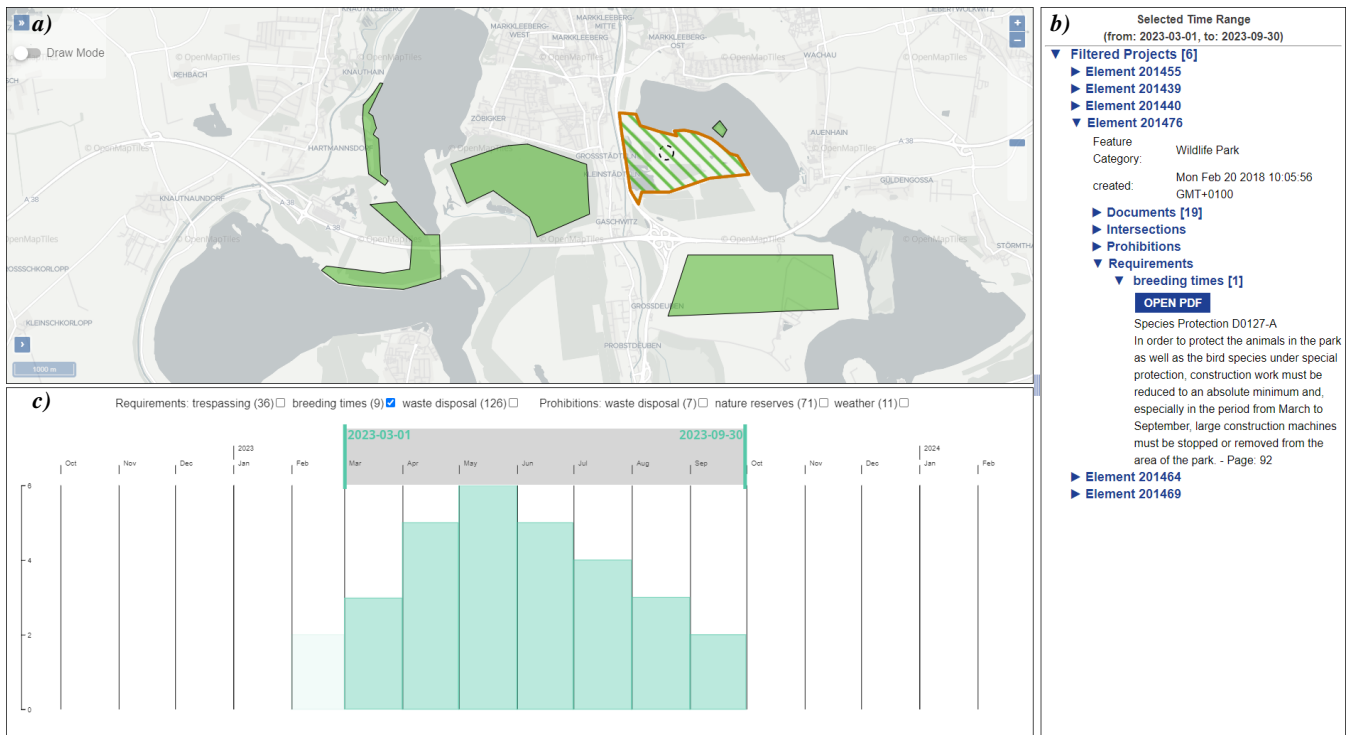
Figure 6: (c) In the timeline view, the documents are filtered according to the displayed region in the map and the Requirement “breeding times”. The time range from March to September was selected. (a) Through brushing, the associated projects of the selected range are displayed on the map. (b) They are additionally listed with further information in the information panel. A selected project states that certain noisy activities are apparently not permitted in the associated wildlife park during the specified time.
