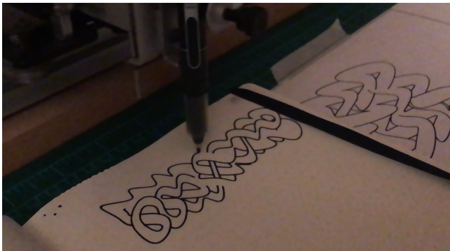
Figure 19: A plotter drawing a pattern generated by our system on a notebook.
