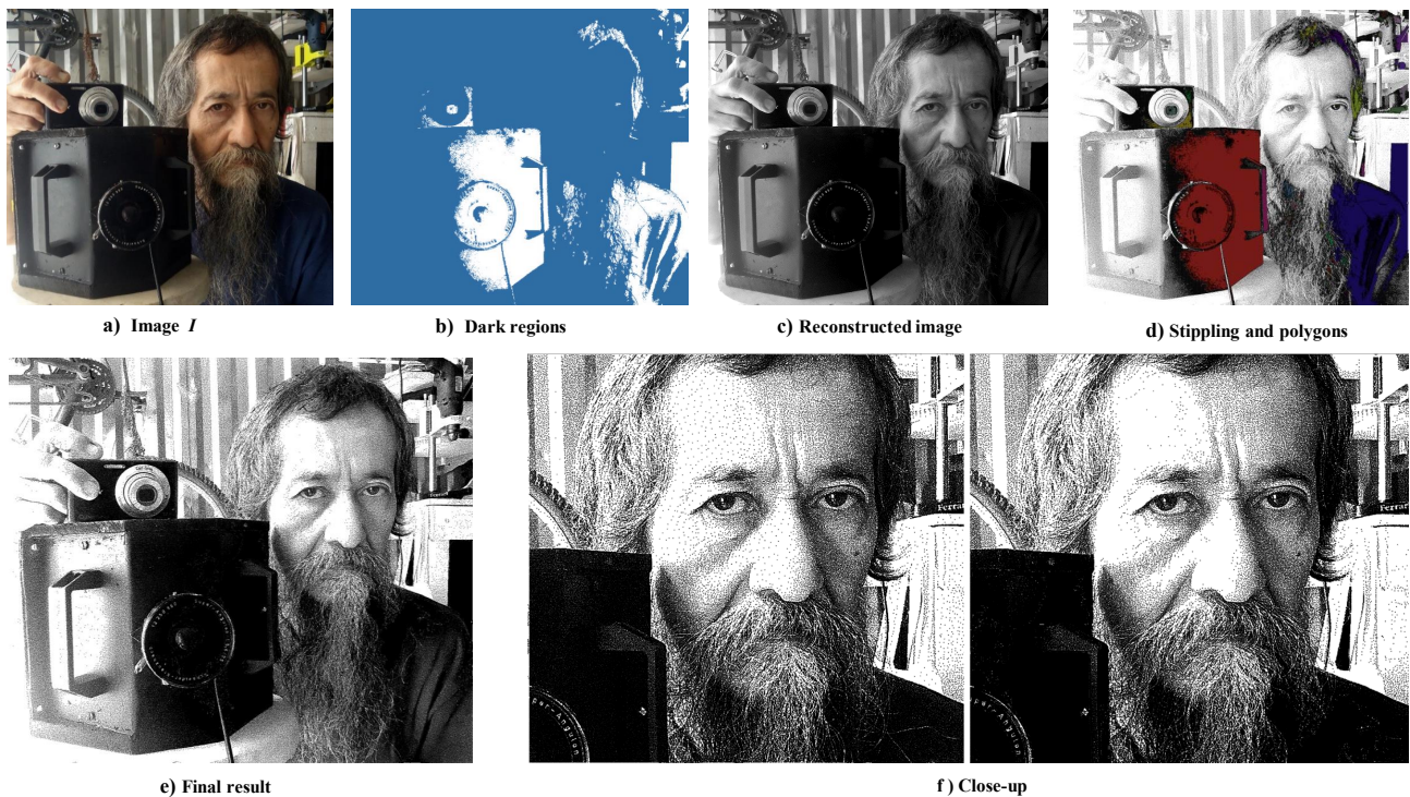
Figure 1: Steps of our method: a) original image; b) threshold mask; c) reconstructed image after Poisson blending; d) results from filling polygons; e) final result after stipple removal; f) close-ups of original stippling and final result of the polygon filling followed by stipple removal steps.
