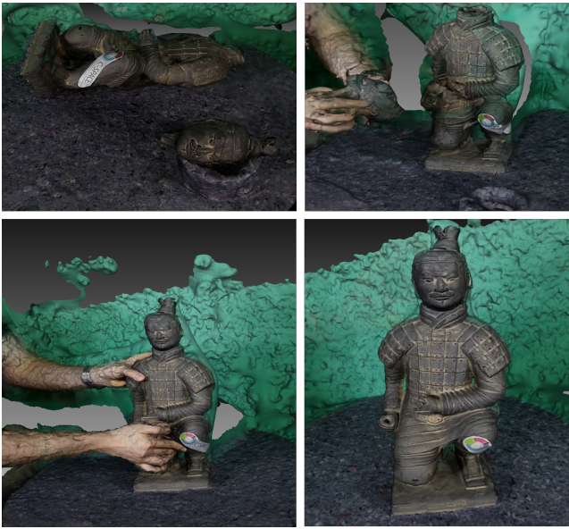
Figure 6: Results of our 4D reconstruction as 3D rendering of four example 4D frames for a cultural heritage artifact, being placed upright and assembled. Time sequence is from left to right and from top to bottom. Input images originate from full HD videos (1920x1080) captured by 12 middle class LG smart phones. Noisy background geometry is due to the lack of image features on a homogeneously colored background.
