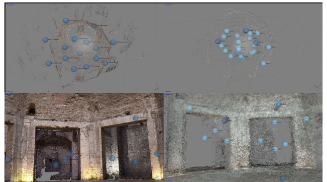
Figure 16: Comparison between tie-points (top) and between dense point-clouds (bottom)
