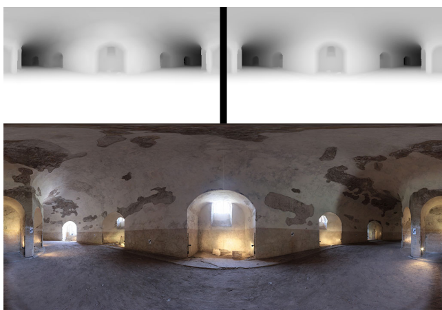
Figure 10: Panorama #3: top row shows differences between computed omnidirectional quadratic depth-map from point-cloud (left) and from mesh-based model (right). Bottom is panoramic color acquisition as reference
