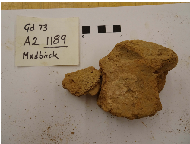
Figure 10: Mudbrick wall samples from Godin Tepe, excavated lot Gd 73 A2 1189. The larger sample on the right has remnants of plastering, a common practice for mudbrick surfaces.
