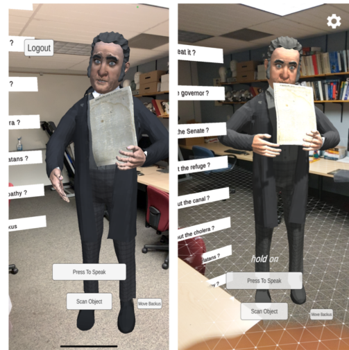
Figure 8: Mobile version of the application implemented for both iOS and Android. The grid indicates a horizontal surface on which the character can be placed. Buttons are used to initiate conversation and to scan objects
