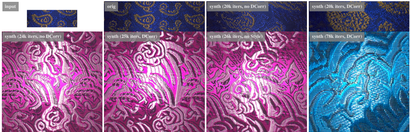
Figure 5: Ablation study for the effect of an additional Deep Correlations term (see Eq. 1). Top row: input, uncropped material, synthesis with style loss only, synthesis with style and deep correlation loss; bottom row (pink fabric): further synthesis results with style loss only, with style and deep correlation loss, and with deep correlation loss only; bottom right (green-blue fabric): typical artifacts observed when using deep correlation loss.
