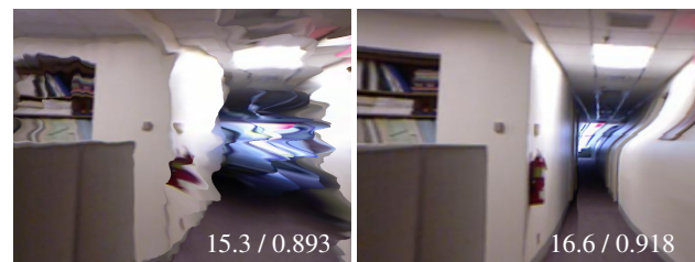
Figure 2: A 3D photograph rendered from a novel viewpoint using depth maps from: the small model with random weights (left) and the trained small model (right). In the bottom right corner of each image are the PSNR and SSIM metrics for those images.
